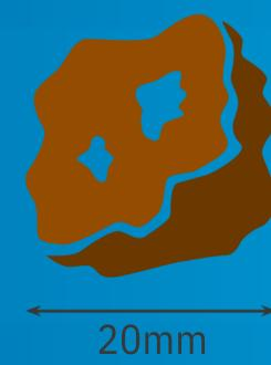
The sub-sample is ground to a particle size of 2mm or less to produce a homogenous sample
