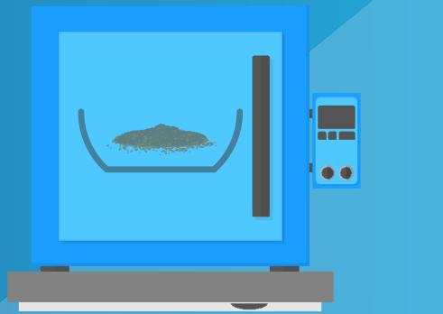
The sample is weighed for the final time. Any organic matter should now be burned off, and the difference between the final weight and its original mass is the Loss on Ignition figure.
