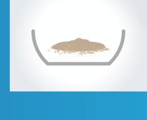
The sample is transferred to a muffle furnace and heated to a temperature of 440°C for a minimum of 5 hours. It is then cooled in a desiccator
