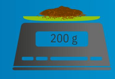
Particles exceeding 20mm are removed and the new weight is recorded
